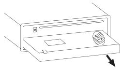
Hold the control panel by its right side and then pull it **straight** out of the bracket.
